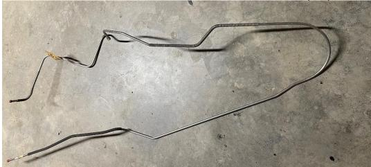
New 1970 Convertible 3/8" stainless steel fuel line from tank to fuel pump. \$50
